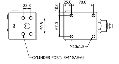
HYTECO EARTHMOVING CRANE VALVE 3/4 " SAE-62 PART NUMBER: HECV12C-SS350-01
