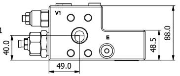
RECOMMENDED WORKING PRESSURE: 350 Bar RECOMMENDED BOLT TORQUE RATING FOR
