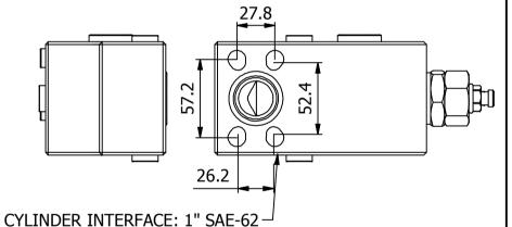
HYTECO EARTHMOVING CRANE VALVE 1" SAE-62
